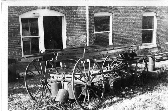
Original Ransom Bucket Wagon currently in the NC Museum of History, Raleigh. Note the ladders and hooks (firemen's pikes) on top & the oil cans to carry water to fight the fires.
